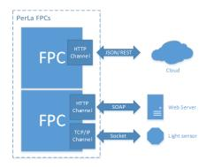
This implementation allows an integration of PerLa with SOAP and JSON/REST services. These technologies could utilized the same Channel despite the REST orientation of HTTP Channel code.
